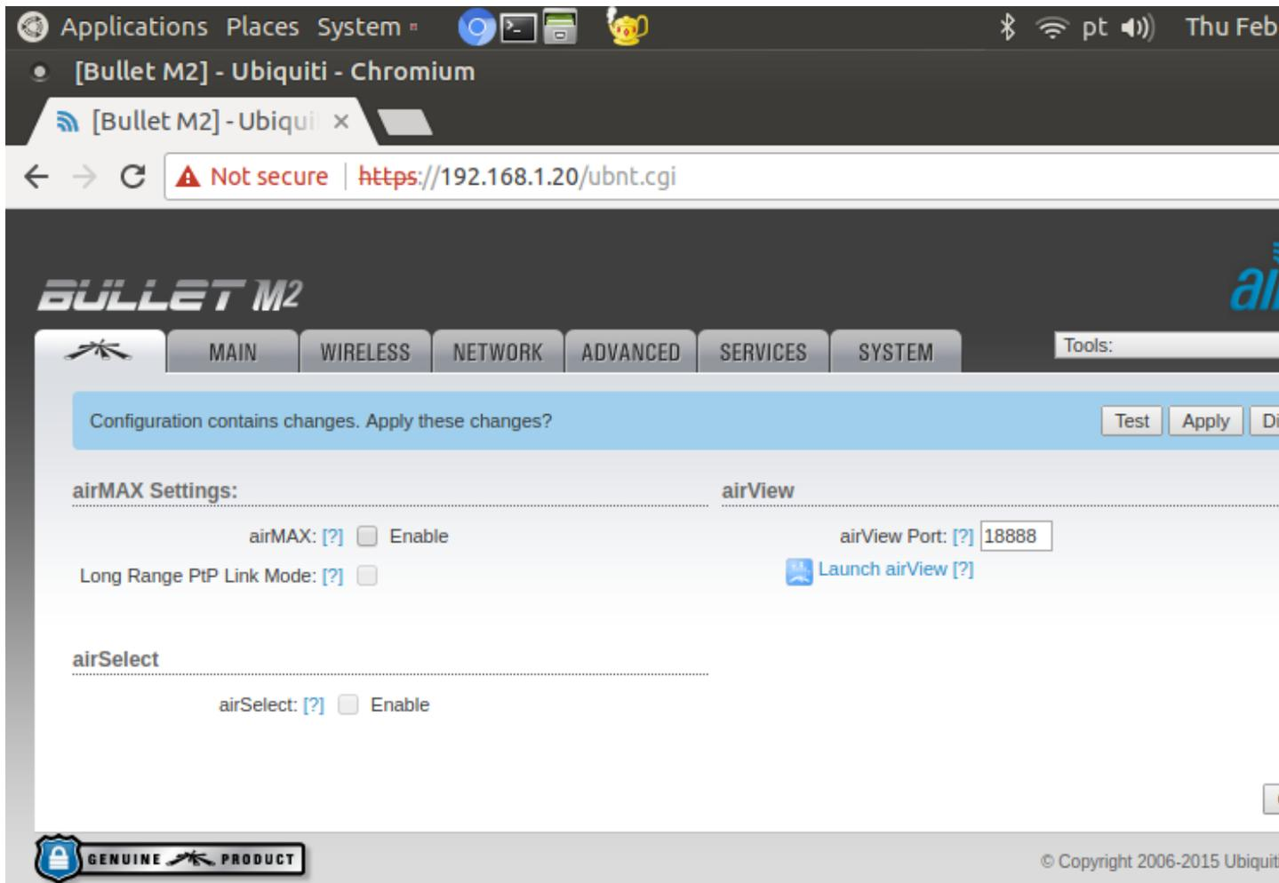
This is sufficient to configure the radio as an Access Point, and it will generate a WiFi network with the specified SSID. However, there are two possible configurations regarding the Bullet’s network role: *Bridge* and *Router* mode.
